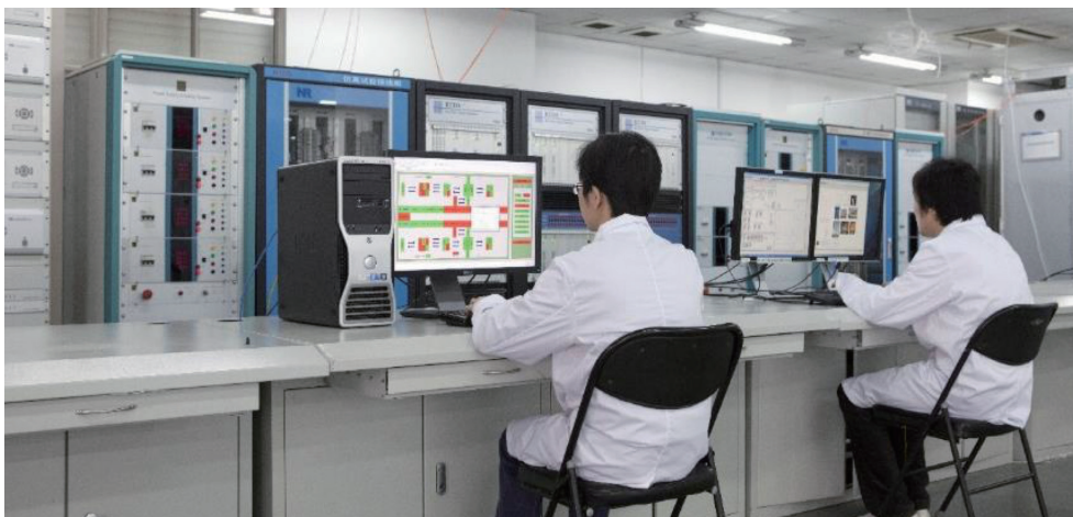
Fig.4 Hardware-in-loop test on RTDs
